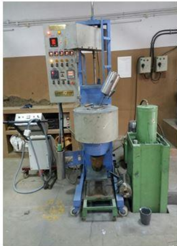
Stir casting 1.7kg Capacity 1000 ° C with squeeze casting, centrifugal and vacuum casting
