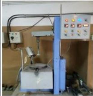
Stir casting 5kg Capacity 1000 ° C
