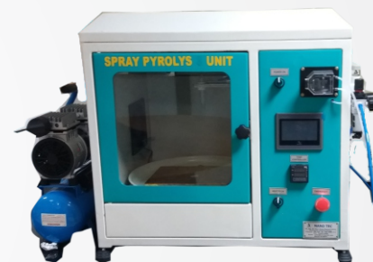
SPRAY PYROLYSIS WITH ULTRA SONIC NOZZLE
