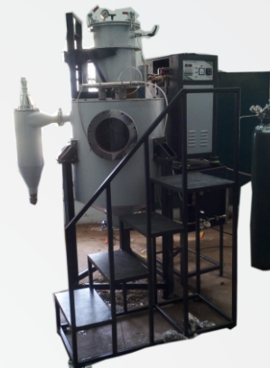
SPRAY PYROLYSIS WITH ULTRA SONIC NOZZLE
