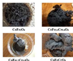
As-prepared condition of pure and \text{Cr}^{3+} substituted \text{CoFe}_2\text{O}_4 magnetic nanoparticles
