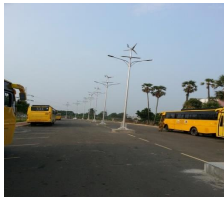
Hybrid type (solar & wind) street lighting
