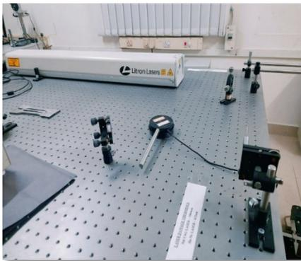
The laser damage threshold (LDT) or laser induced damage threshold (LIDT) is the limit at which an optic or material will be damaged by a laser given the fluence (energy per area), intensity (power per area), and wavelength. LDT values are relevant to both transmissive and reflective optical elements and in applications where the laser induced modification or destruction of a material is the intended outcome.
