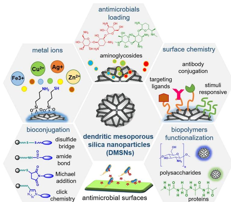
**Figure 1.** Diagram summarizing the key surface functionalization techniques for DMSN in the preparation of efficient antimicrobial materials.
