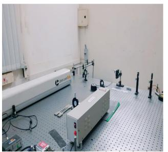
**Specifications:** Litron Lasers Nd-YAG Laser Energy - 400 mJ Laser Wavelength - 1064nm Pulsed duration - 6ns
