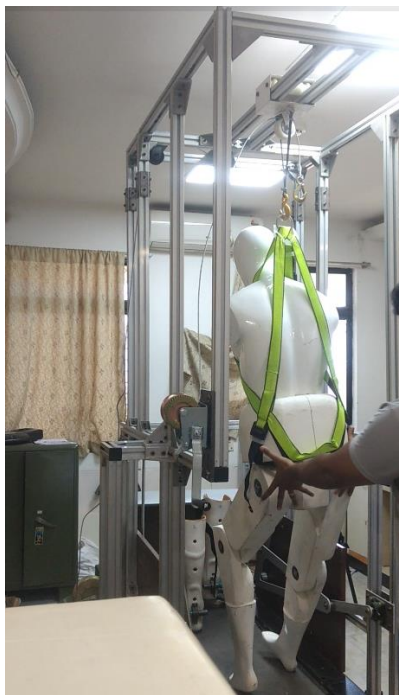
Fig. 1 Trial of the Lifting and transfer mechanism
