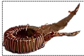
**Fig. 1 Image of Tunable Inductor**
